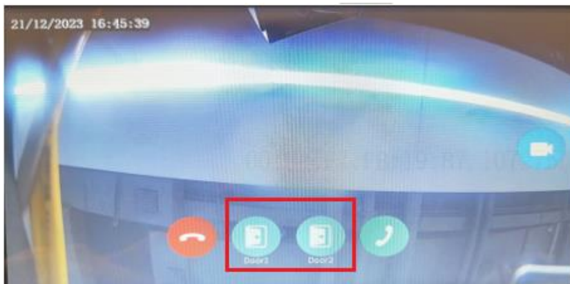
Figure 4-35 Multi-Lock Configuration Screen on Door Station
