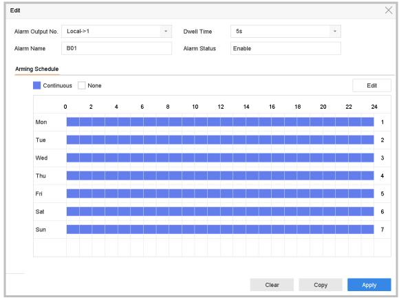
Figure 11-12 Alarm Output
