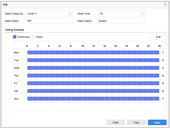
Figure 11-9 Alarm Output
