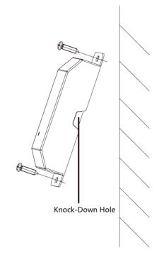
Figure 4-3 Install Secure Door Control Unit
