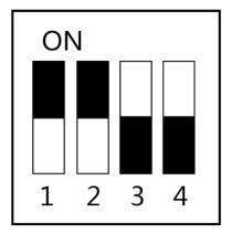
Figure 4-2 DIP Switch (Binary 0011)
