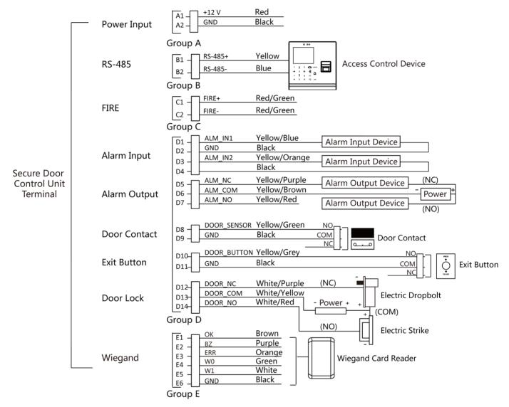
Figure 3-1 External Devices Wiring Description
