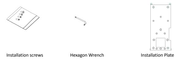
Step 2: Fix the plate to desk bracket with screws (36mm screw hole), then put device onto plate, fix with device bottom screws.
