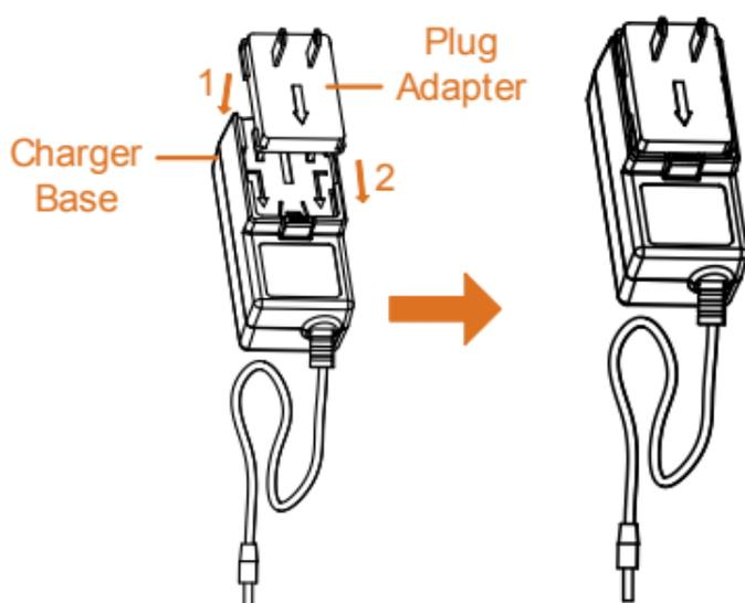
3. Connect the power adapter to the battery charger.
