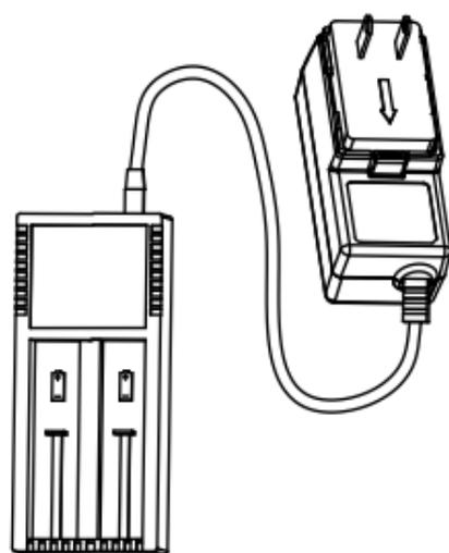
4. Insert the batteries in the charger with positive/negative terminals corresponded.
