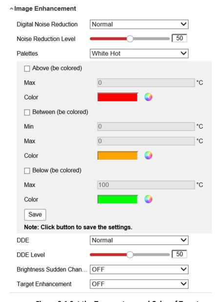
Figure 9-1 Set the Temperature and Color of Target
