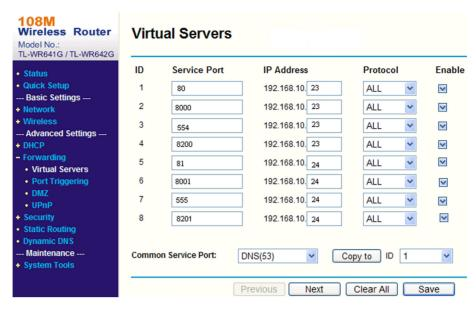
Figure 9-1 Port Mapping on Router
