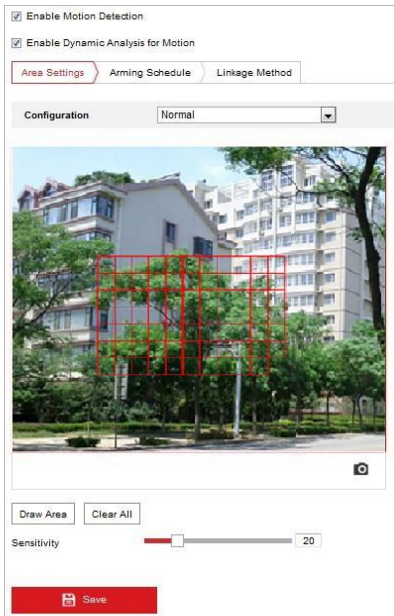
Figure 5-9 Motion Detection Settings-Normal
