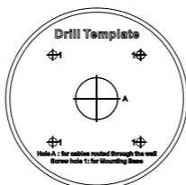
Figure 2-9 Drill Template of the Junction Box
