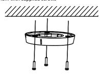
Figure 2. 6 Attach the Mounting Base to the Ceiling
