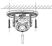
Figure 2. 11 Attach the Mounting Base to the Ceiling
