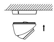
Figure 2. 7 Secure the Camera with Mounting Base
