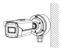
Figure 2-13 Combine the Junction Box's Cover with its Body
