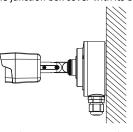
Figure 2-7 Fix the Junction Box Cover back to its Body
