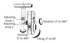
Figure 3-12 Adjust the Camera
