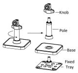
Figure 3-6 Disassemble the Bracket
